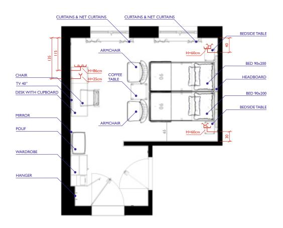
All symbols determine the middle of the socket/frame. The height H indicates a dimension between the axis of the socket/frame and finished floor. Horizontal dimensions are being counted from walls to the axis of the socket/frame.
