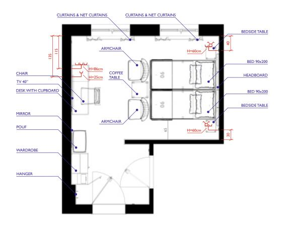
All symbols determine the middle of the socket/frame. The height H indicates a dimension between the axis of the socket/frame and finished floor. Horizontal dimensions are being counted from walls to the axis of the socket/frame.
